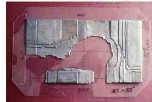
Fig. 1. How a compensator was constructed from thin lead sheets glued together in order to modulate the intensity of a tangential beam for improving the homogeneity of dose in breast radiation therapy (Courtesy of the Breast Technology Group, Royal Marsden NHS Foundation Trust)
