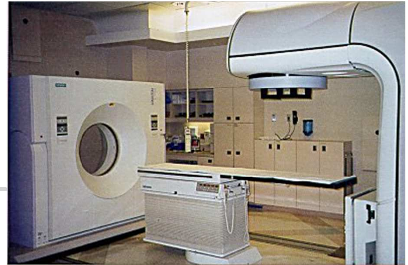
With the PRIMATOM System, the gantry holding the CT scanner encircles the patient on the treatment table. During scanning, the gantry moves incrementally along high-precision rails, providing updated tumor localization data. The gantry retracts when scanning is complete.
