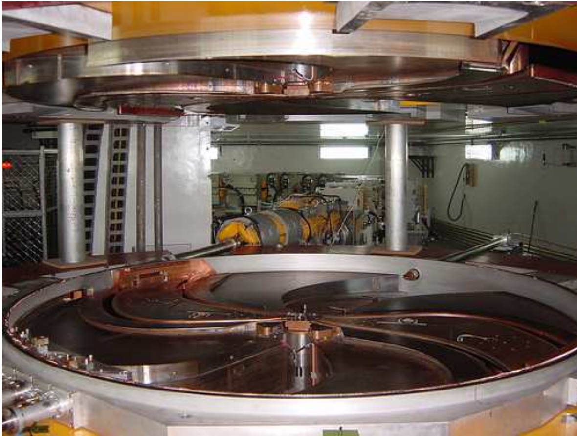
Hydrogen plasma ion source inside of the accelerator
