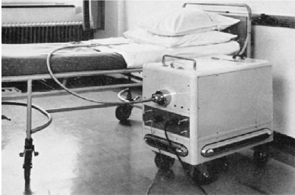
Figure 3. Illustration of early single-channel remote afterloading system (Walstam 1962). An LDR source train at the end of a flexible cable was used to move the source to and from the patient to a shielded safe under control of an automatic timer. A radiation detector was used to verify source position.
